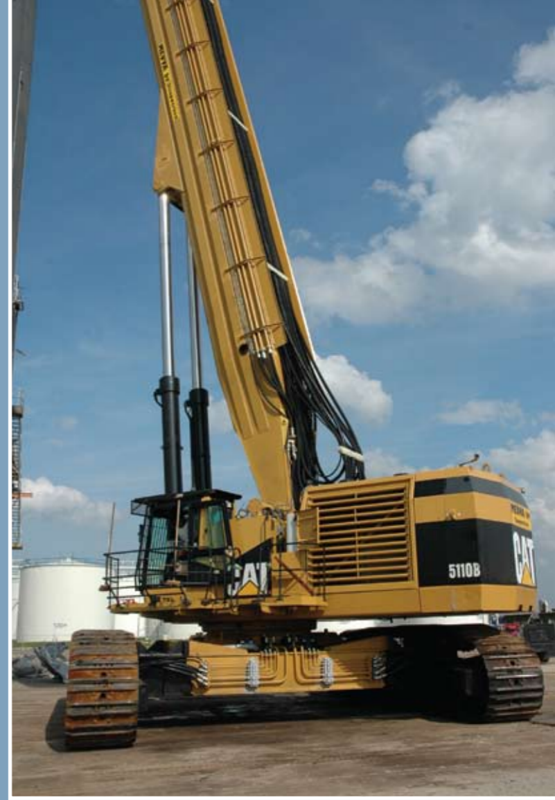
Above: Made in Dubai, each of the main lift cylinders weighs 4.5 tonnes. When fully extended they have a length of 12m.
