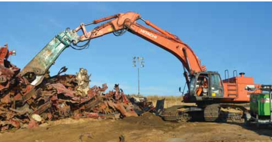
The huge metal chunks stripped from the wreckage are cut into manageable pieces by a Hitachi ZX470 with a 4.3-tonne scrap shear.
